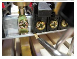
When spacing wippens, use a mirror to watch the jack tenders, and also verify that the wippen heels are centered on the capstans.
