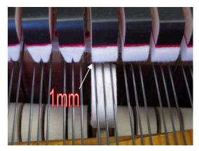
For easy hammer spacing, put 1mm shim (metal ruler) between keyframe and action stop block
