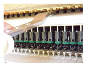
With the 1mm ruler in place, adjust the left edge of hammer to be even with the left string.
