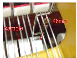
Once sample hammers are set, slide action out and regulate the capstan screws in the remaining hammers to form a straight line.
