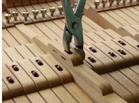
Lift up the Key back 1-2mm and release. It should fall down slowly by its own weight, without sticking. For best results, key should fall more slowly in dry conditions, and a little faster during humid conditions.
