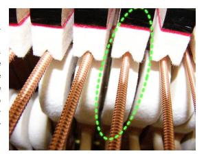
The contact point of the hammer is centered under the bi-chord strings.
