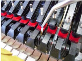
To position the jack tender under the let-off button, insert traveling paper underneath the side of the wippen flange that you want the jack to move towards.
