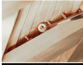
Square the keys so that the top surfaces are horizontal, by tapping the balance pin side to side.
