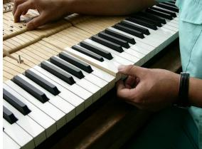
Easing a tight front hole bushing using key pliers
