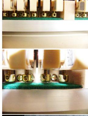
The head and pedal lever should have lost motion of 1-2mm at the damper lever.
