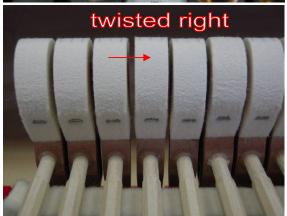
Checking hammer angle – spaces between hammers must be equal and parallel at the "rest" position.
