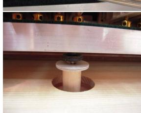
Adjust pedal rod head to set the sample damper levers so that they start moving when the hammer is 23mm (1/2 blow distance) from string.
