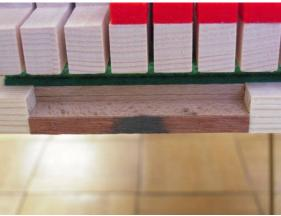
If most hammers are aligned towards the left from strings, glue a shim (wood veneer or thick paper) to the back side of Action Block.
