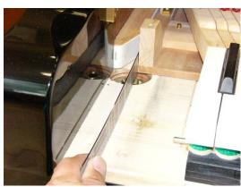
Use the Hammer flange spacer under the pin block while looking down between the strings.
