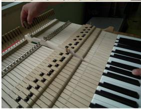
If the key sticks then ease the balance hole. This process must be done carefully until the key moves with the desired ease, but is not too loose.
