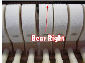
Place a piece of travel paper between the flange and hammer rail on the same side of the screw as the direction the hammer is traveling. Differences in thickness or length of paper will determine the degree of correction.
