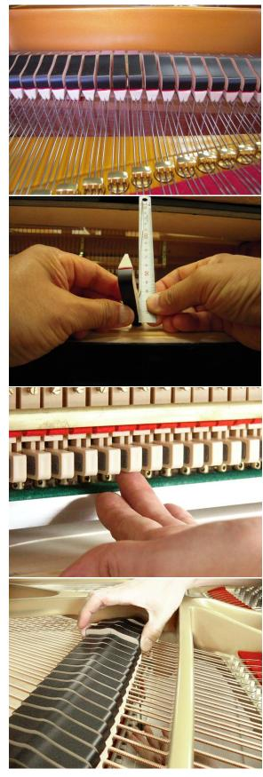
Loosen all damper block screws, and adjust damper lever capstan to make the damper levers same height. Place a ruler on top of the damper levers as shown to assist in adjusting the capstans.
