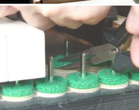
Black keys should be about 2mm higher than white keys, when black keys pushed down to bottom.
