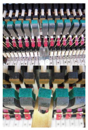
Set backchecks on white keys so the hammers check 15mm from the strings on a medium mf blow.
