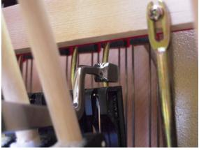
Lift by Key: Damper should lift with the key when hammer is halfway through its travel. Bending the damper spoon toward the strings causes the damper to lift earlier; toward the action causes later lift.
